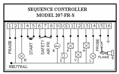
Note: It is important to connect Burner body to the Controller Ground at Terminal 16.
