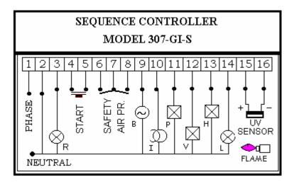
The Outputs are relay contacts, with a rating of 230V AC, 5A resistive. However, the Controller total output current should not exceed 5A and is protected by a 5 A fuse.
